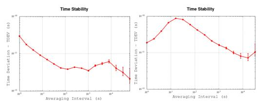
TDEV comparison for TTA and WR transfers over 180 km of field deployed fibre
